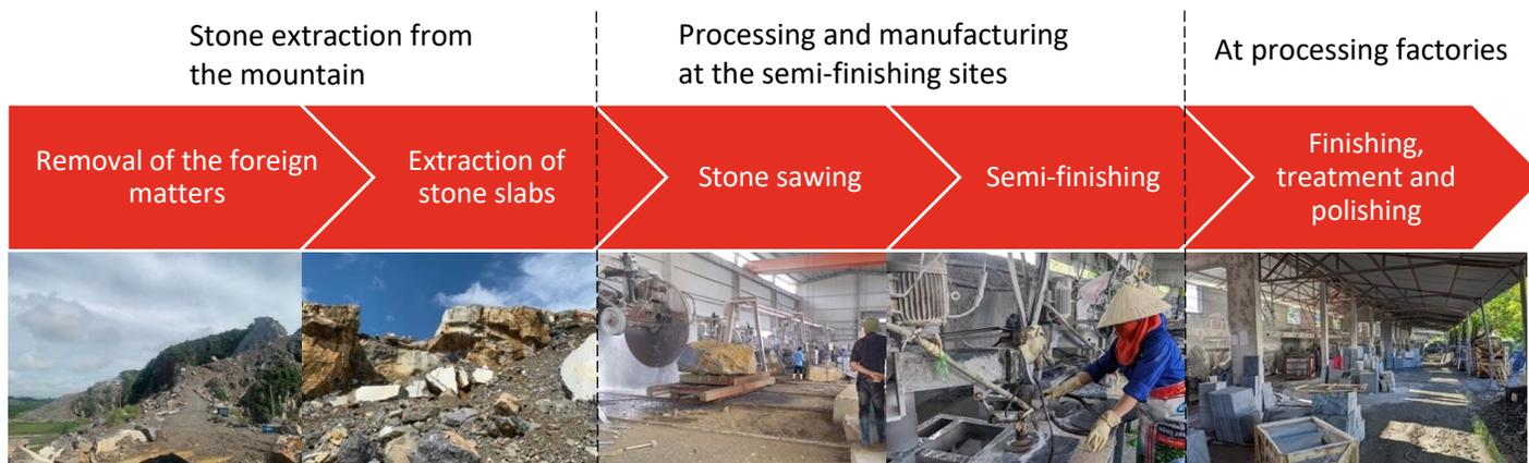
Appendix 4 provides details about bluestone producing phases, including extraction, processing and transportation.
